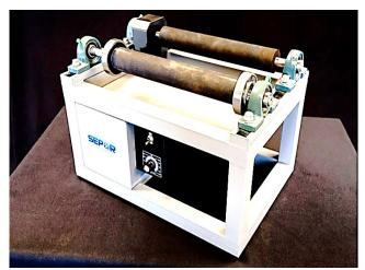
AC electric input is converted to DC for speed control in a 20 to 320 RPM range. The distance between rolls is also variable. A wide variety of jar sizes can be used. All units are operable on 50 or 60 Hz.110 V/1 Ph/60 Hz or 220 V/1 Ph/50 Hz.
