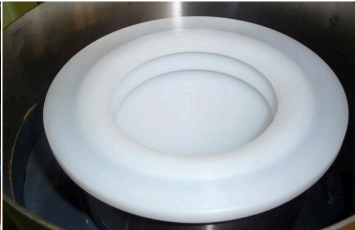
The centrifuge's bowl, high SG solids are held in the ring area, against the wall, while light solids exit with water.
