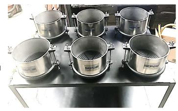
filter plate, with two hand lug attachments for holding the 10 inch diameter by 6 inch height steel cylinder body firmly in place. The filter sits on legs that elevate it from the bench. A package of 100 each high wet strength filter papers and one filter cloth with 25 micron pore openings is included with each filter. The filter will hold up to 2 gallons of slurry.
