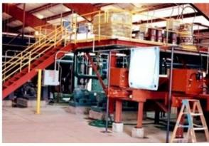
The vacuum system removes oxygen from the solution in a packed tower. Solution is percolated through a packing bed while under a
