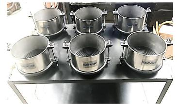
filter plate, with two hand lug attachments for holding the 10 inch diameter by 6 inch height steel cylinder body firmly in place. The filter sits on legs that elevate it from the bench. A package of 100 each high wet strength filter papers and one filter cloth with 25 micron pore openings is included with each filter. The filter will hold up to 2 gallons of slurry.
