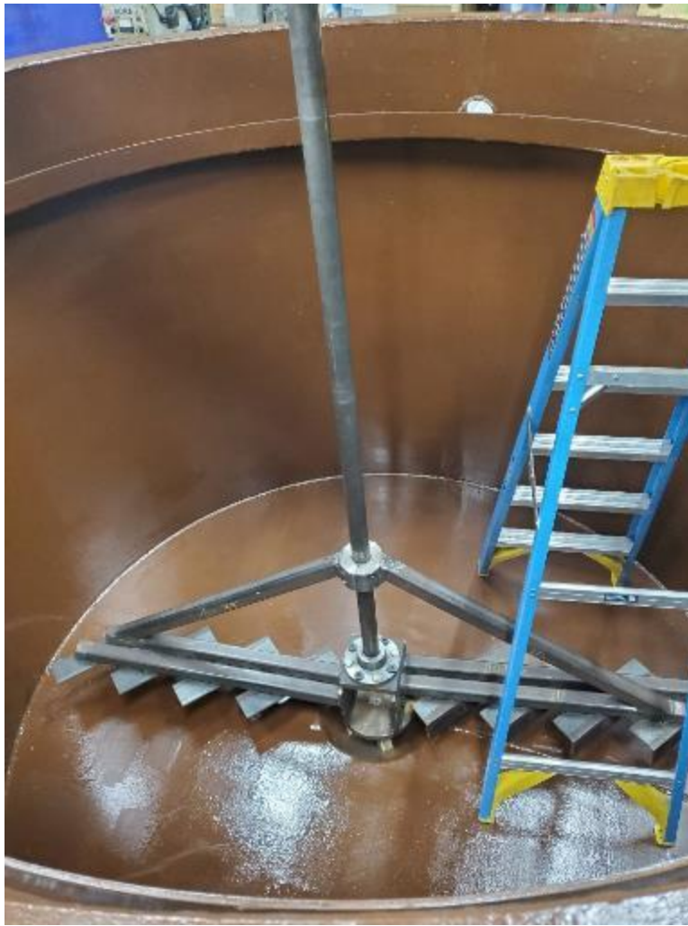
Thickener with acid and temperature resistant coating
