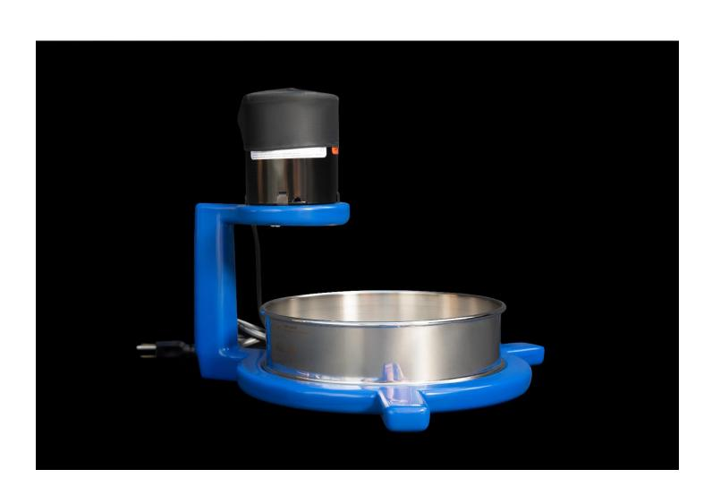
The Sepor Wet-Dry Sieve Shaker is supplied for the purpose of conducting relatively simple size analysis for materials. The sieve shaker uses standard 8 inch diameter laboratory sieve screens and has a capacity for 2 full height 8" diameter sieve screens.
