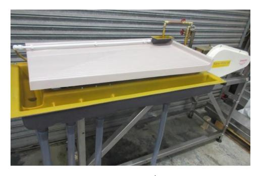
This lab scale unit is good for handling up to 50 kg/hr on a continuous basis or can be used to process 1 kg samples at a rate of up to 20 per hour. It is available in 110V or 220V versions and requires about 3 gpm of wash water. The deck is 0.8 m² in area. It comes with two gel coat decks, for fine or coarse sample processing and has a five outlet launder with two splitters. It comes with a water spray gun for dilution, and stroke, tild and end slop are adjustable while in operation.
